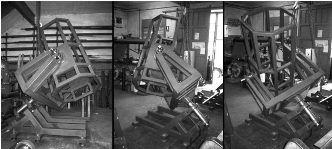
Figure 9: Bulding the new mountings: All tubular structure: simple, easy, light and low cost
