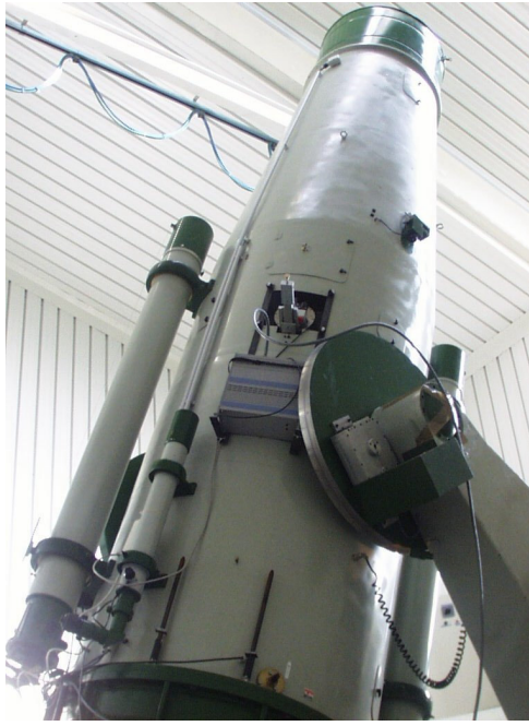
Fig. 1 – The SCAM camera head and its electronics attached to the NW side of the S/67-92cm telescope at Cima Ekar.
