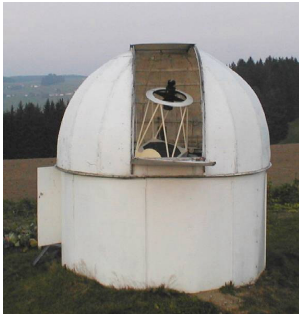
Figure 1: The Davidschlag Observatory at dusk. The 0.6m f/3.3 reflector is visible inside the 4.5m plastic dome.
