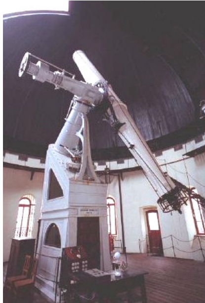
Figure 3: View of the 27" Grubb Refractor at Vienna. Image courtesy Vienna University Observatory.
